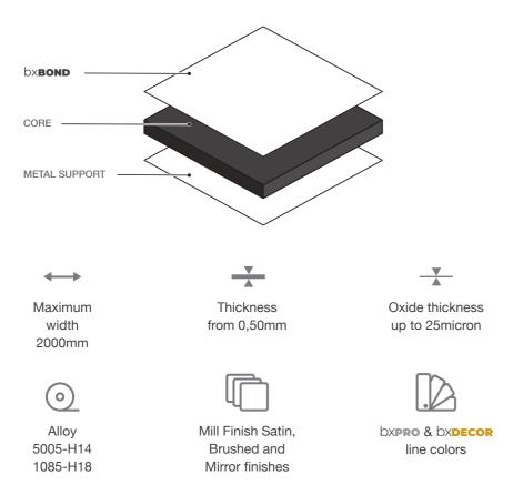
Due to its low thickness, bx**BOND** is ideal for being combined with other materials and suitable for the production of composite panels.
